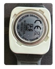
This picture shows what the rear of the falls detector looks like, it does not have a missing cover and is safe and ready to use.
